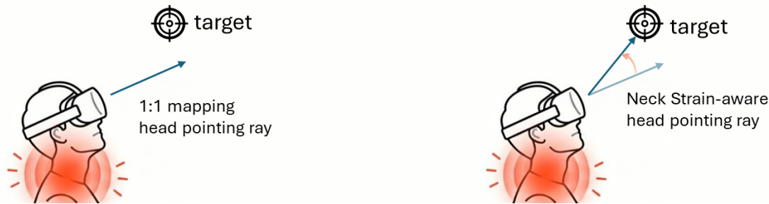
Figure 1: Strain-aware head pointing. Left: 1:1 mapping head pointing cannot reach the target, and neck strain occurred. Right: Neck strain drives the cursor and amplifies the pointing ray angle, enabling target acquisition.
